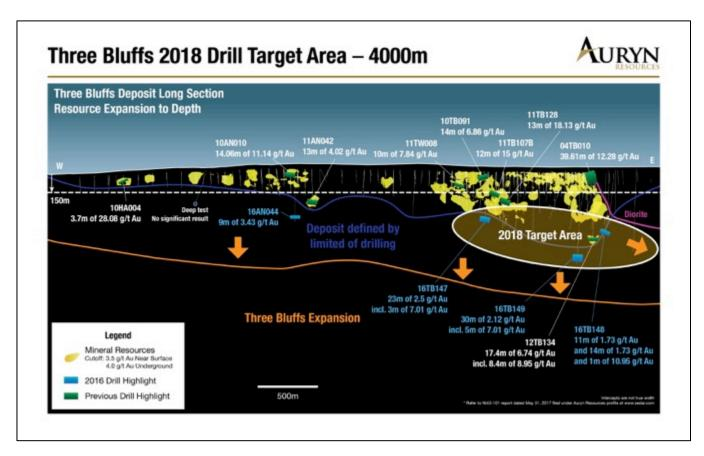
Figure 2: Illustrates a long-section of the Three Bluffs deposit with the target area for the spring drill program highlighted. The drill program has two goals; to expand the resource and to explore for previously unrecognized mineralized zones to the northeast.
