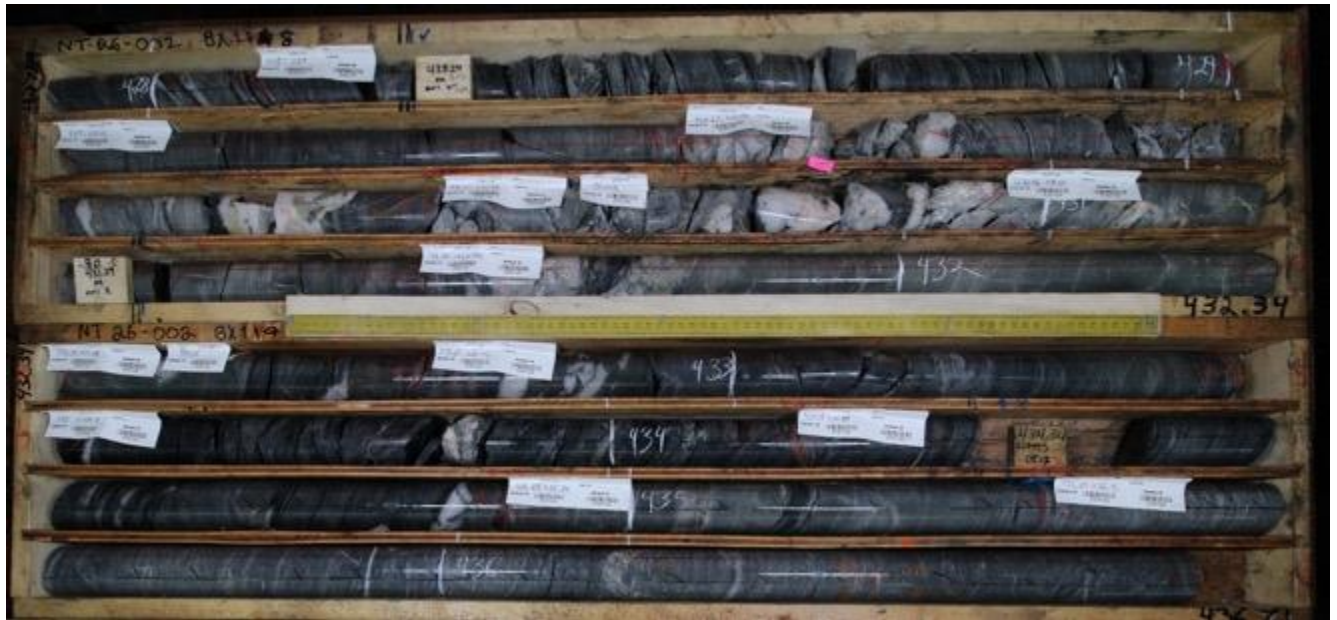
Figure 12: Quartz extensional vein in NT-26-002, hosting visible gold (Figure 13), pyrite, and bismuth sulphosalts. While visible gold can be an indicator of grade for an interval, due to the variable nature of nuggety gold, presence of visible gold may not always indicate high-grade assay results.
