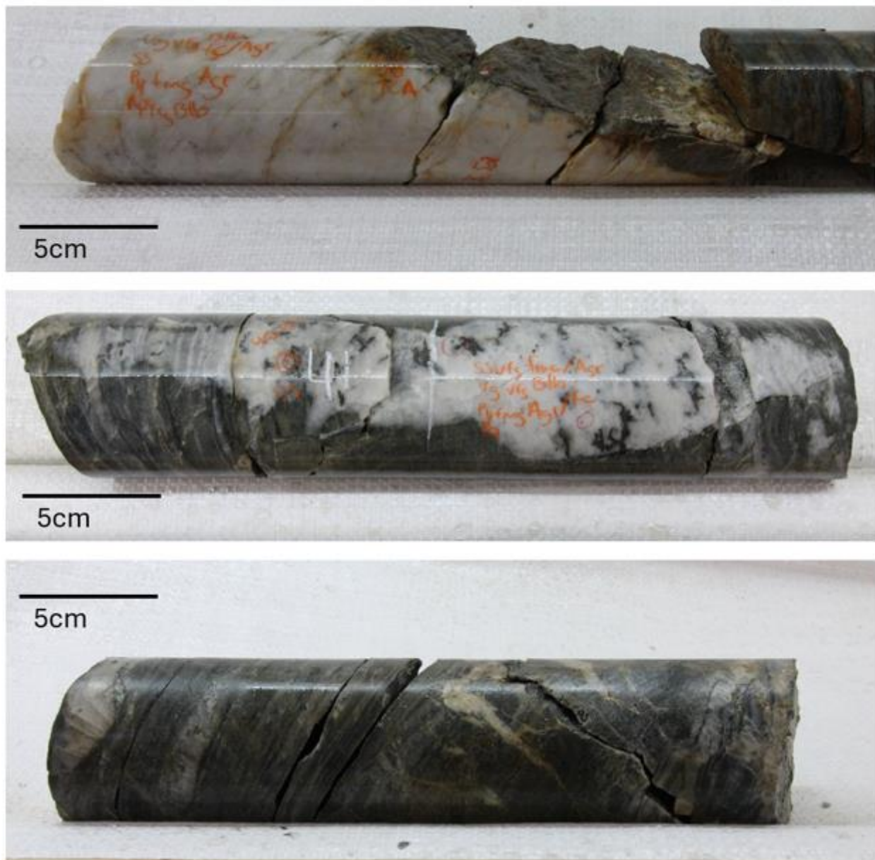
Figure 5: Potential mineralized intervals from drillhole NT-26-006: Top - 36.2-36.7m – extensional quartz vein bearing visible gold, bismuth sulphosalts, arsenopyrite, and pyrite. Middle – 40.9-41.2m – extensional quartz vein bearing visible gold, bismuth sulphosalts, pyrrhotite, and pyrite. Bottom – 41.9-42.2m – local quartz shear veins and extensional quartz-carbonate veins associated with calc-silicate alteration and pyrrhotite, arsenopyrite, pyrite sulphide replacement of calcareous metasedimentary rocks.
