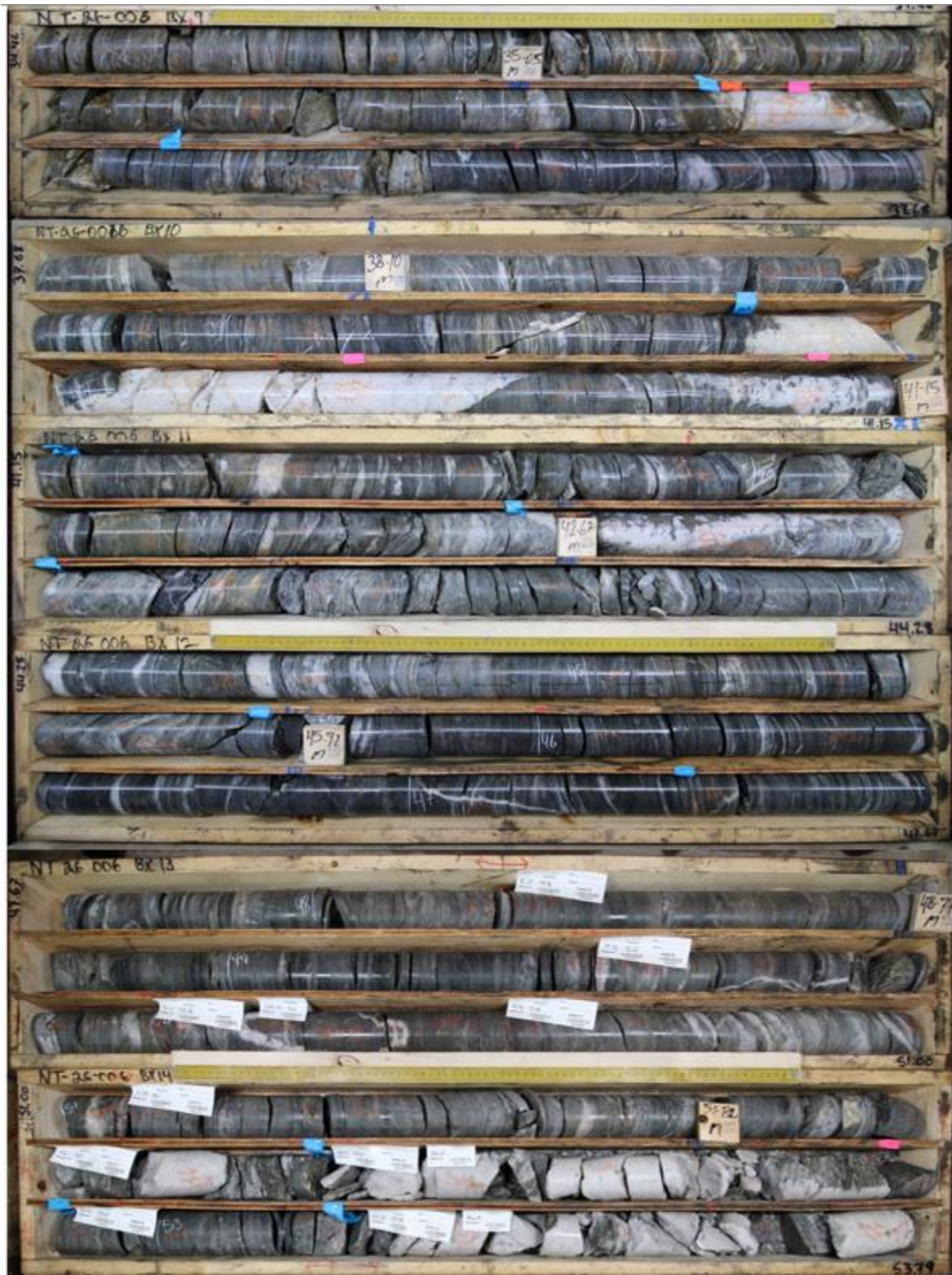
Figure 4: Mineralized extensional quartz veins in predominantly metasedimentary rocks in drillhole NT-26-006 from Nitra. The Quartz veins host visible gold, bismuth-sulphosalts, and arsenopyrite (Figures 5 and 6).
