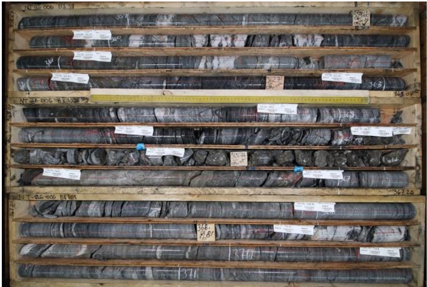
Figure 9: Zones of brecciated and annealed rock in drillhole NT-26-006. Healed breccias and associated shear zones may be indicative of long-lived, large structures, which can act as fluid pathways for regional mineralizing systems.
