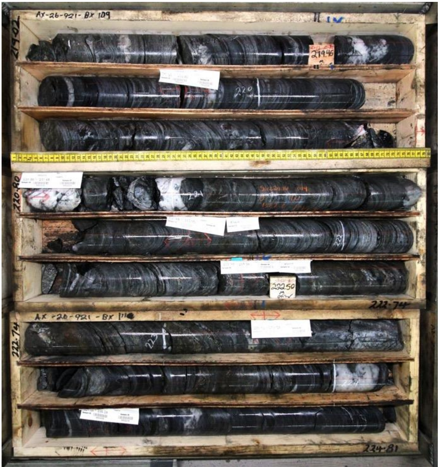
Figure 5: Intersections from drillhole AX-26-921 depicting sulphide replacement in high-grade intersections down-dip of main Airstrip zone (see cross-section in Figure 3).
