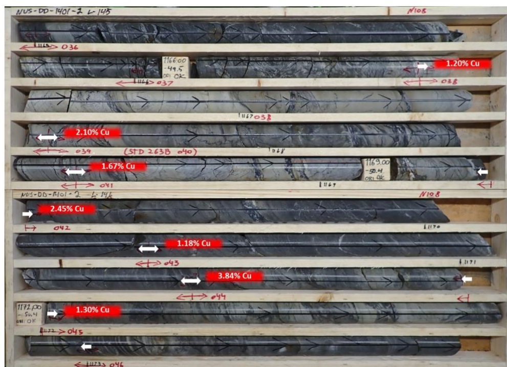
Figure 2, Mineralized drill core from NUS-DD-1401-03A showing the brecciated dolomite horizon encompassed within the local schists. Sample values (copper) are marked in red whilst the white arrows mark the sample boundaries
