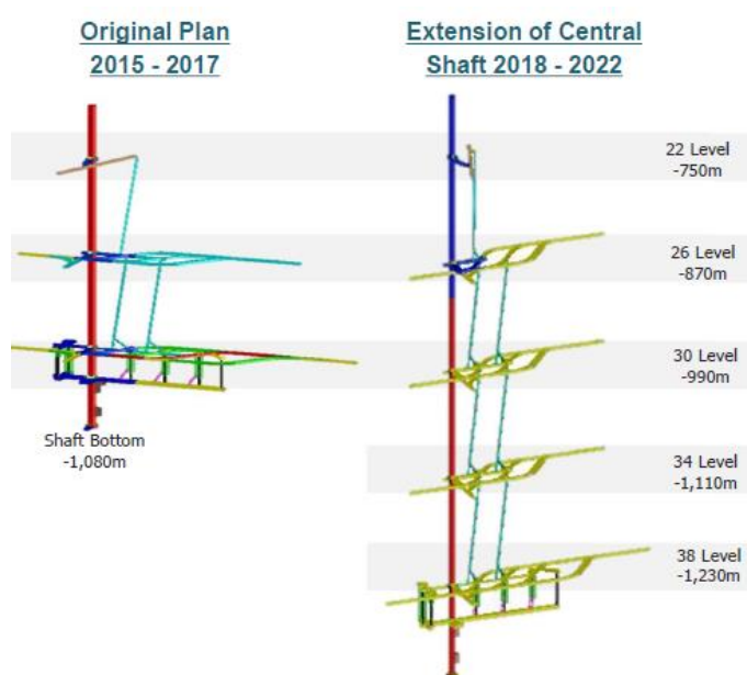
Figure 7: The new plan for the Central Shaft
