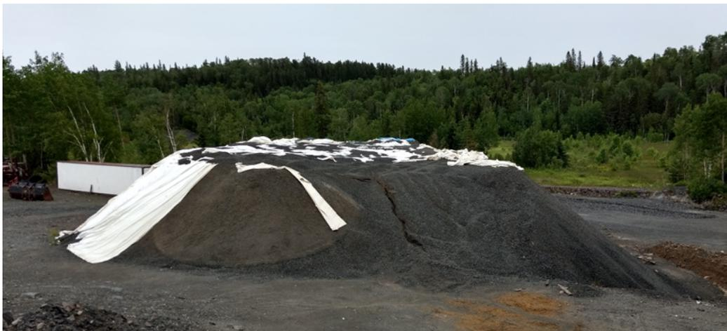
**Image 1. Pile of crushed waste rock material at First Cobalt mill site.**
