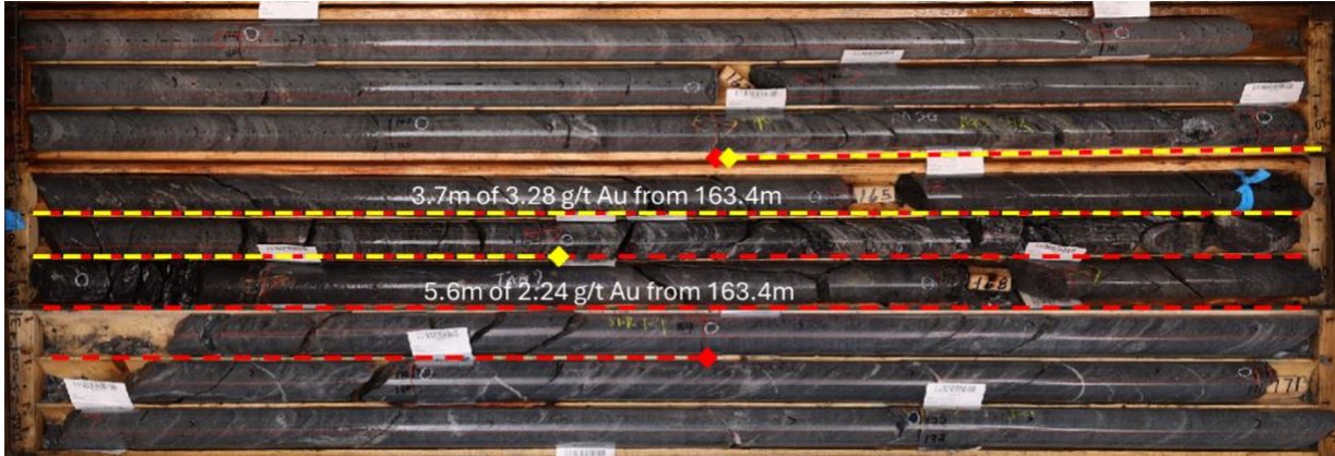
Figure 3: Hole DBD-25-001: Sheared metasedimentary rock horizon containing exhalative pyrite and strongly sheared graphitic argillite beds with deformed quartz-carbonate veins returning an intersection of 5.6m of 2.24 g/t Au from 163.4m, including 3.7m of 3.28 g/t Au from 163.4m.
