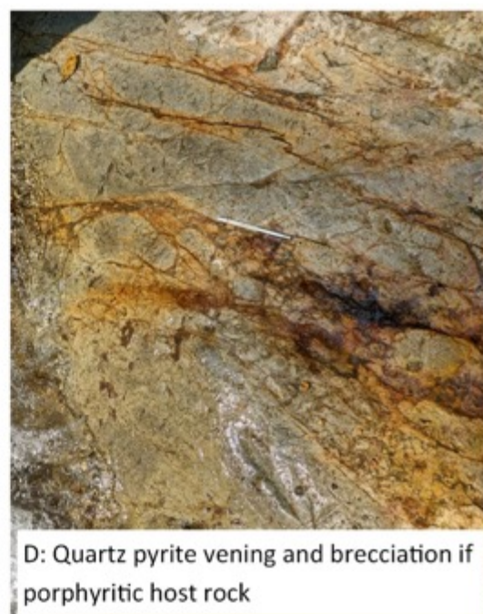
Figure 4 Rock photos from Divisoria showing outcrops of hydrothermal brecciation and quartz-pyrite veining. The area is exposed for 300m before it disappears under cover.
