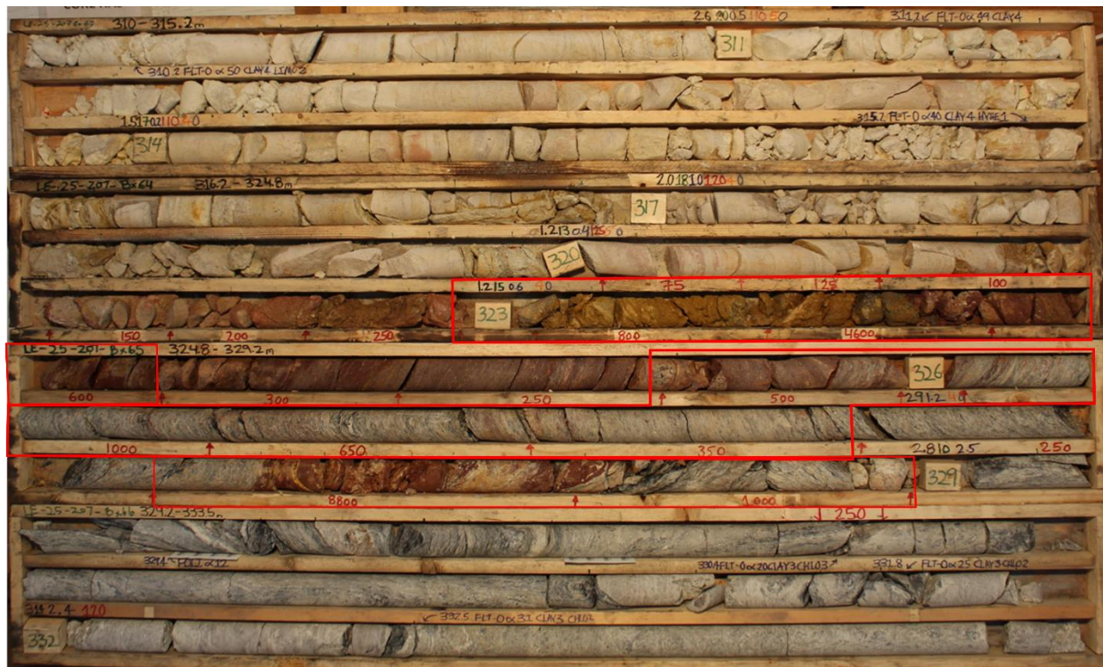
Figure 5 – South Trend: Core photo of drill hole LE25-207 from 310 m to 333.5 m showing interval from 323.0 m to 329.0 m with elevated radioactivity up to 8800 cps averaged over 50 cm on the RS-125 spectrometer. The unconformity is at 323.8 m.
