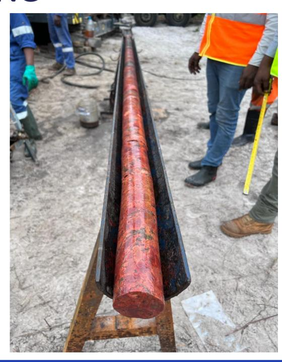
Stage 1 drill programme is in progress with the extension of historic drillhole BA002 now coring beyond the bottom of the old hole at a depth of 1 approx. 519m
