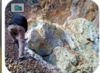
RC21903, channel sampling of 6m-wide structure with adv. Argillic alteration. Pyrite, enargite, copper oxides 1m channel sample at 0.53 g/t Au, 17.5 g/t Ag, 861 ppm Cu, 6.8 ppm Mo
