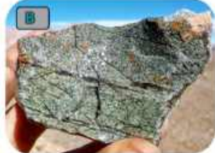
RC21930, Quartz veinlets in sericite alt diorite. Au: 0.50 g/t, Ag: 0.3 g/t, Cu: 356 ppm, Mo: 9.2 ppm
