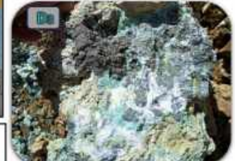
RC21902, select sample of Pyrite - enargite + copper oxides from structure in D1 Au: 0.97 g/t, Ag: 14.7 g/t, Cu: 0.36%, Mo: 5.9 ppm
