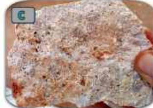
RC21886, Residual quartz-vuggy silica with adv. argillic alteration, silica = alunite, 1.5m at 0.86 g/t Au, 22.1 g/t Ag, 51.7 ppm Cu, 17.2 ppm Mo, 115 ppm Sb
