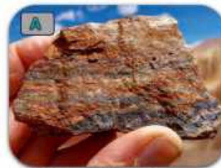
RC21893, Quartz veinlets ± sul. Au: 0.75 g/t, Ag: 1.3 g/t, Cu: 354 ppm, Mo: 41.8 ppm
