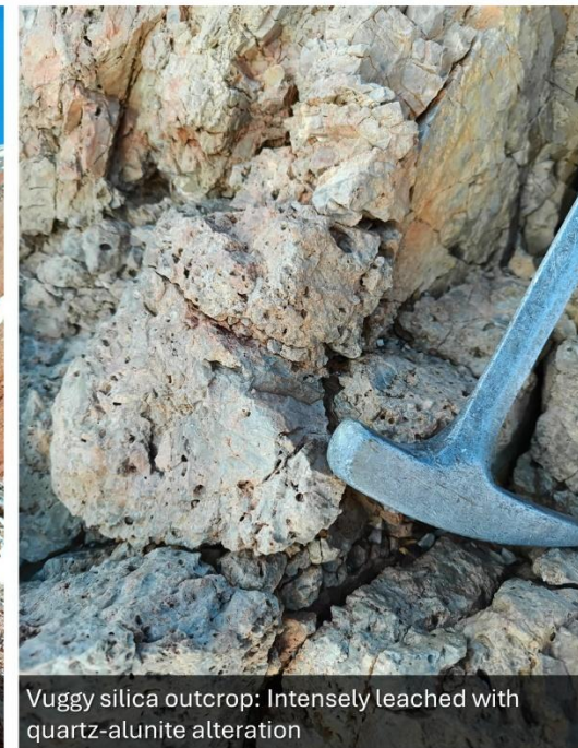
Meseta: Hydrothermal breccia, intense quartz- alunite alteration, clasts of vuggy silica, strong leaching
