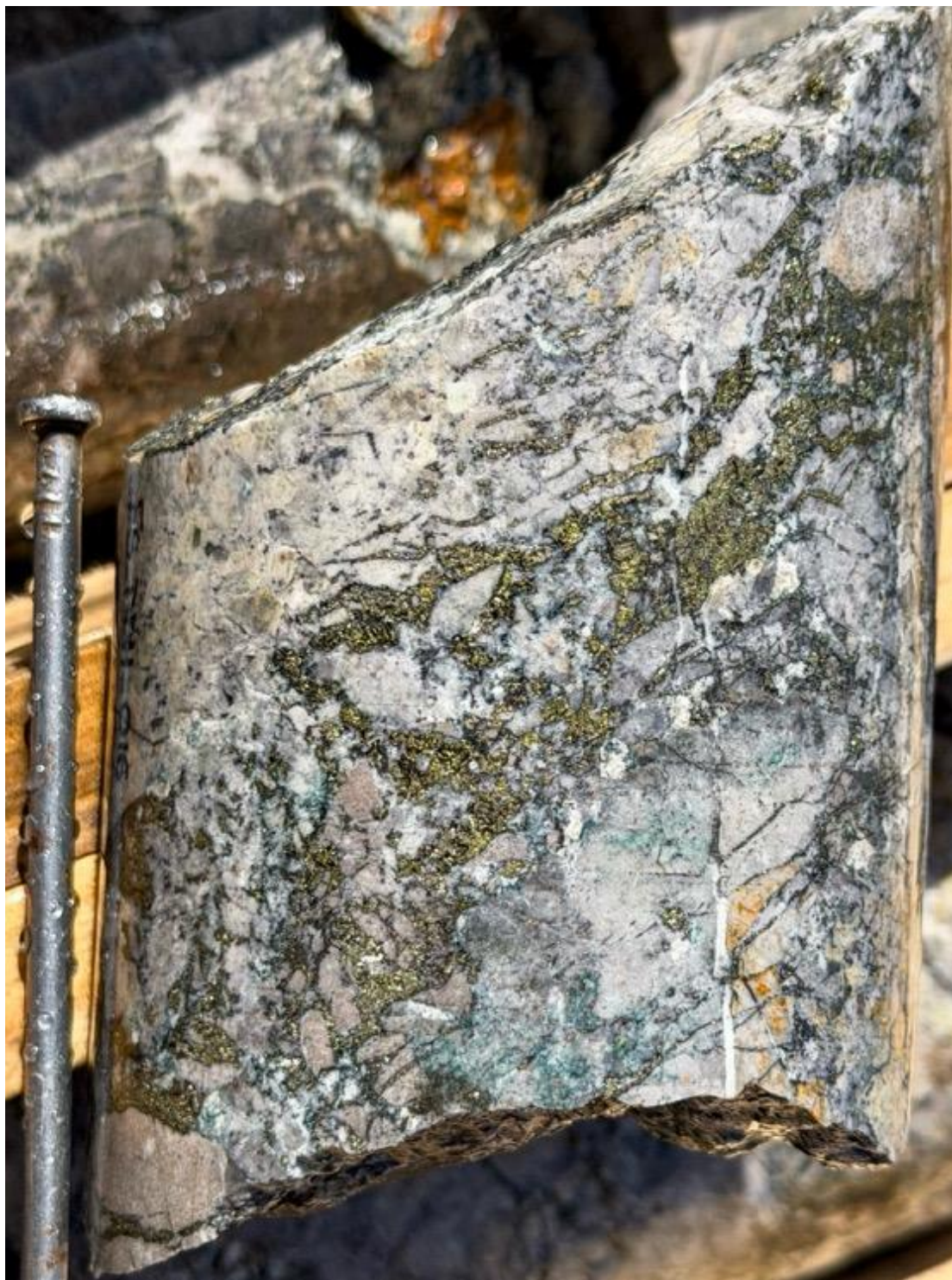
Figure 1: Core from 125.75m (FS_DD016), 125-126m assays at 1.67% Cu, 1.62 g/t Au, 1.69 g/t Ag, 685 ppm Mo
