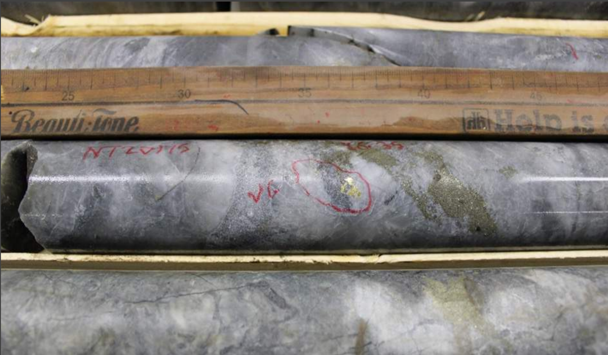
Visible Gold clot in Drill core hole NT20-175
